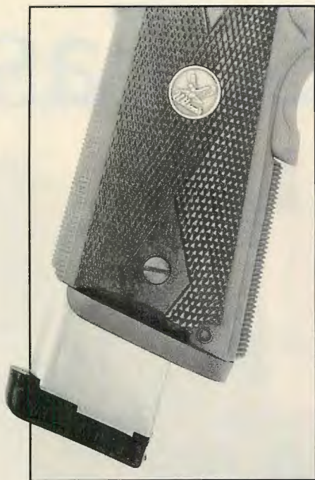
Special Ops CQB's front strap and mainspring housing feature EDM-cut checkering. Other features include Wilson exotic-wood, checkered grip panels and the Wilson-Rogers eight-round magazine.
